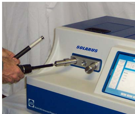
figure 10 Loading TEM holder, holder adapter, and plug
