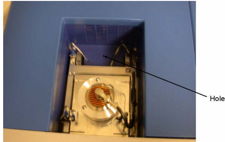
figure 24 Access to Pirani gauge calibration button
