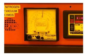
Check the HMDS fill level and vacuum inside the vacuum flask, on the left side of the tool. Pressure inside the flask should be < -85 kPa (-25 in. Hg).
