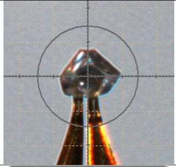
16. Exit the mounting window and close the cabinet. Click the small arrow next to "Screening." Set theta=-35, exposure time about 2-5 seconds. Click "Ok & Screen."
