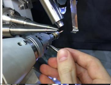
**14.** Rotate to phi=90 and adjust the crystal left/right again.
